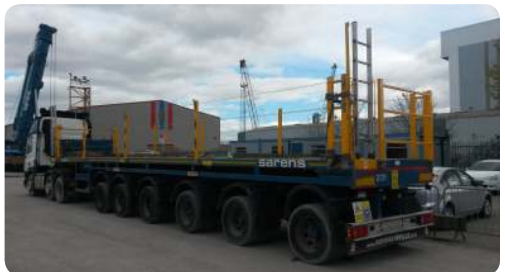
Safety guards on trailers used as a tool in prevention (working on height) at Sarens UK
