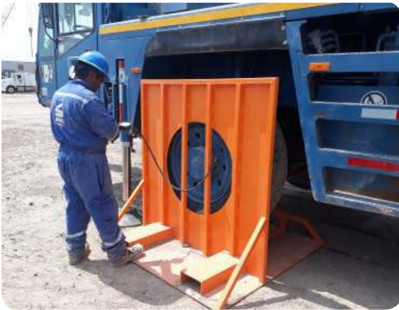
Using a tire inflation cage for safe working in Mexico
